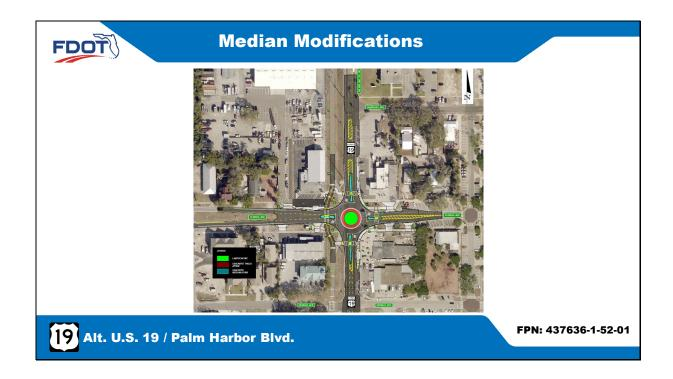
The roundabout will include raised concrete medians/islands on the north and south entrances to the roundabout on Alternate U.S. 19 and on the east and west entrances on Florida Avenue.
