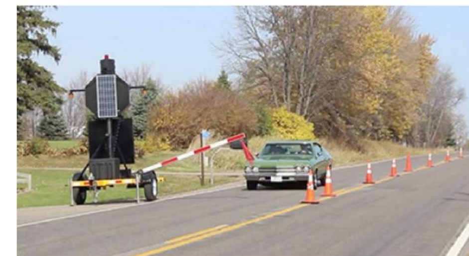
AUTOMATED FLAGGER ASSISTANCE DEVICES (AFAD) ARE TEMPORARY TRAFFIC CONTROL EQUIPMENT.
